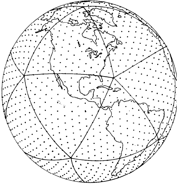
FIG. 1. Spherical geodesic grid used for computations reported in this paper.
